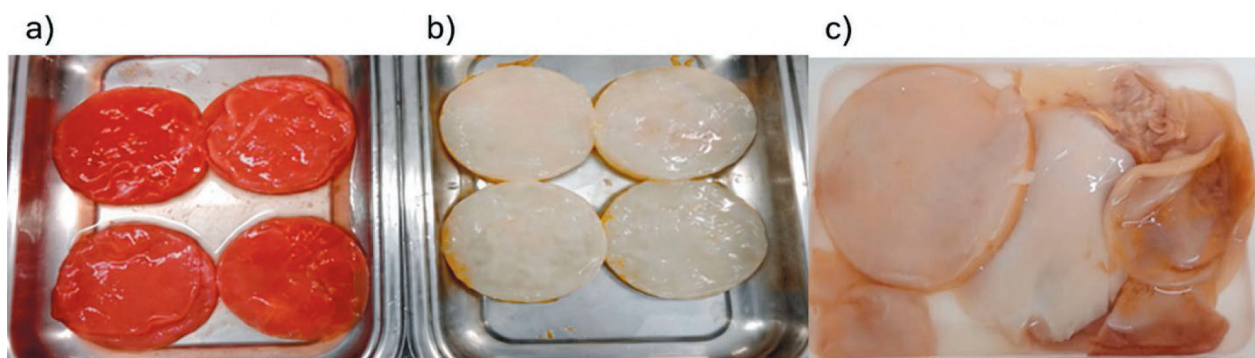
Fig. S2. Obtaining bacterial cellulose from: a) acerola, b) passion fruit, and c) green tea substrate
