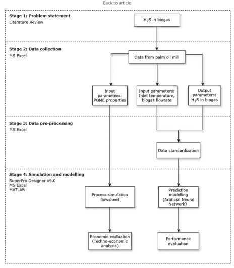
Fig. S1. Framework for simulation and prediction modelling using machine learning and economic analysis. POME=palm oil mill effluent
