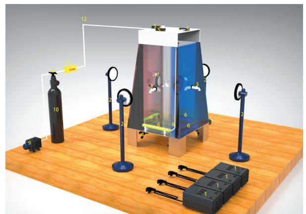
Fig. 1. Experimental set-up of novel pyramid photobioreactor for *Chlorella* sp. cultivation: 1=power supply, 2=external light source, 3=sampling valves, 4=discharge valves, 5=air intake, 6=sparger, 7=internal light source, 8=air tubing, 9=air pump, 10=CO<sub>2</sub> reservoir, 11=syringe filters, and 12=connecting pipe
