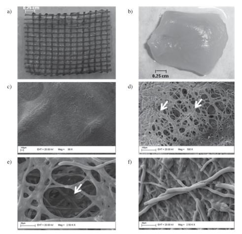
**Fig. 1**. Polyethylene inert support (a) used to produce *A. phoenicis* biofilm (b). SEM microphotographs showing the morphological pattern of the biofilm structure (c) with the spaces and channels among the hyphae (d and e) and hyphal elongation (f) after 72 h of fermentation
