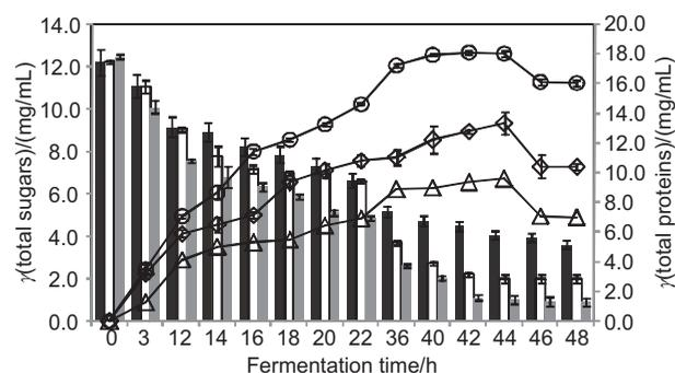
**Fig. 2.** Substrate utilization plot of *B. amyloliquefaciens* at various aeration rates in parallel fermentor system. Substrate utilization (■) and total protein (○) levels at 1.0 vvm in bioreactor C; substrate utilization (□) and total protein (◇) levels at 0.5 vvm in bioreactor B; substrate utilization (■) and total protein (△) levels at 0.2 vvm in bioreactor A
