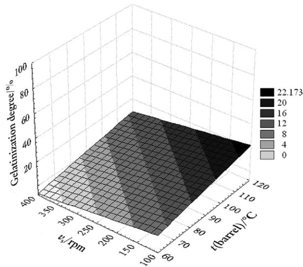
**Fig. 7.** Starch gelatinization degree as a function of barrel temperature and screw speed
