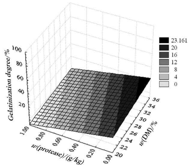
**Fig. 9.** Starch gelatinization degree as a function of the mass fraction of GA protease and dough moisture
