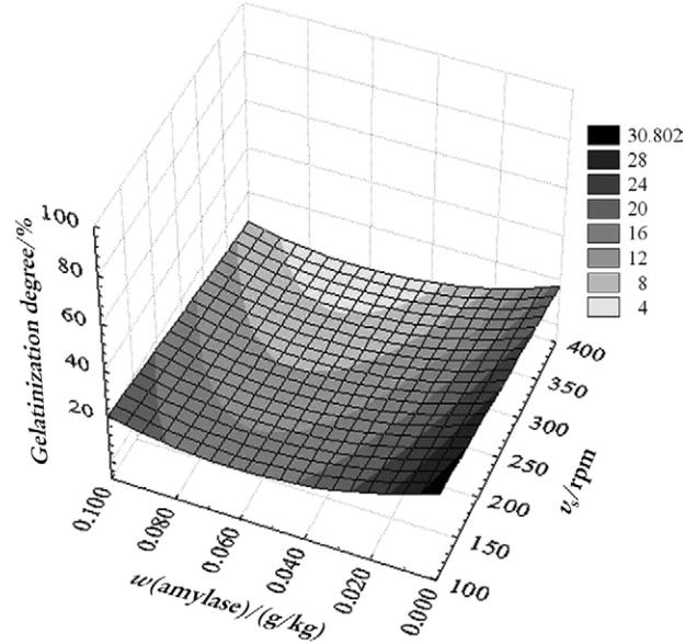
**Fig. 8.** Starch gelatinization degree as a function of the mass fraction of GA amylase and screw speed
