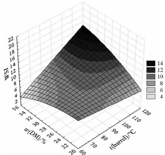
Fig. 2. Water solubility index (WSI) as a function of barrel temperature and dough moisture (DM)
