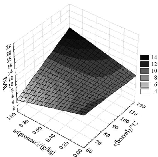
**Fig. 4.** Water solubility index (WSI) as a function of the mass fraction of protease and barrel temperature
