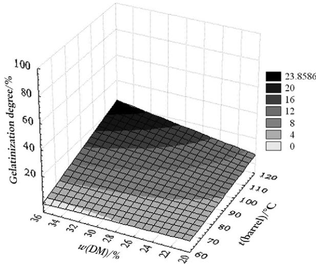
**Fig. 6.** Starch gelatinization degree as a function of barrel temperature and dough moisture
