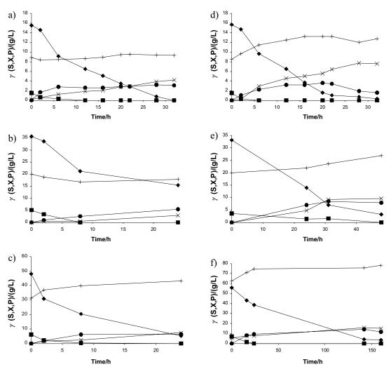
Fig. 2. Bioconversion with *D. hansenii* NRRL Y-7426 of media obtained by autohydrolysis-posthydrolysis, detoxified by charcoal adsorption and concentrated in various initial xylose concentrations. a), b), and c): experiments in media supplemented with yeast extract, malt extract and peptone (YMP medium). d), e) and f): media supplemented with corn steep liquor (CSL). Symbols: xylose ( $\blacklozenge$ ); xylitol (x); biomass (+); ethanol ( $\blacklozenge$ ); glucose ( $\blacksquare$ ).
