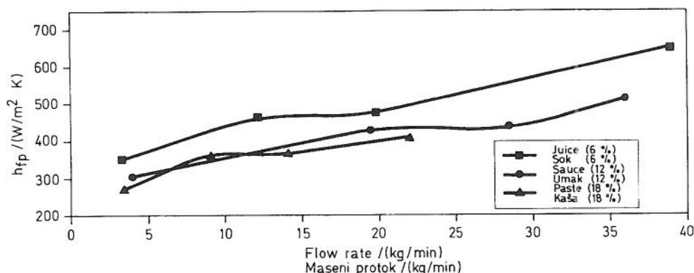
Fig. 1. Estimated values of  $h_{fp}$  vs. fluid mass flow rate for the tested products
