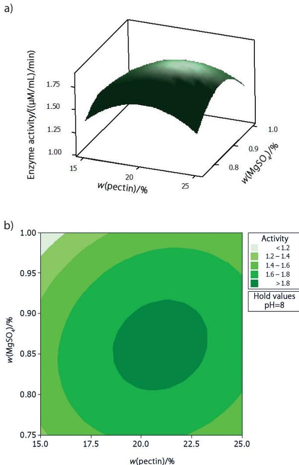
**Fig. 4.** Surface (a) and contour (b) plots showing the effect of interactions of MgSO<sub>4</sub> and pectin mass fractions on pectinase activity
