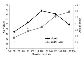
Fig. 4. Effect of the reaction time on oil extraction yield and acidity index
