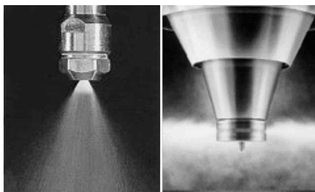
Fig. 3. Pressure nozzle and rotary nozzle, respectively. Reprinted from: GEA Process Engineering Inc. (31)
