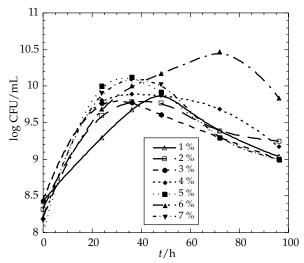
Fig. 1. Effect of CSS concentration on *Serratia marcescens* WF count during 96 h of fermentation at pH=6.5 and 28  $^{\circ}$ C. The symbols indicate different concentrations of CSS
