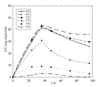
**Fig. 4.** Effect of pH on *Serratia marcescens* WF extracellular specific units (UC) of chitinolytic activity during 96 h of fermentation at 6 % of CSS and pH=6.5. The symbols indicate different pH
