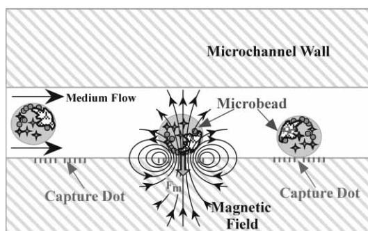
Fig. 1. Microchannel type biosensor. Transport and capturing of microcapsules containing immobilized chromatophores within the magnetic field generated by »capture dot«
