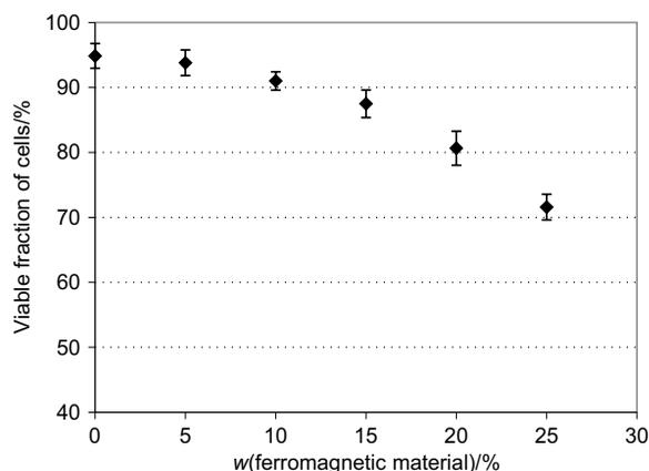
Fig. 3. Effect of the amount of ferromagnetic material in gelatin beads on chromatophore viability. Reaction conditions: L-15 medium supplemented with 5 % serum, pH=7.4, time  $t=140$  min, stirring rate  $v=40$  rpm, cell/bead ratio  $\lambda=70$ . Data presented are mean values of 3 experiments  $\pm$  standard deviation
