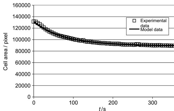
Fig. 5. Decrease of the cell area of immobilized chromatophores with time, as a response to clonidine ( $c=50$  nM). Experimental data ( $-\square-$ ), and model data ( $-$ ),  $\sigma=0.009$  %
