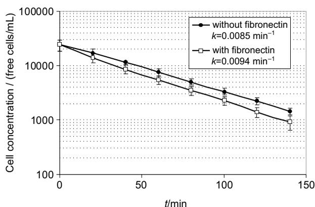
Fig. 2. The kinetics of the attachment of fish chromatophores on gelatin microcarriers with 10 % of iron(II,III) oxide. Reaction conditions: L-15 medium supplemented with 5 % serum, pH=7.4, time  $t=140$  min, stirring rate  $\nu=40$  rpm, cell/bead ratio  $\lambda=70$ . Data presented are mean values of 3 experiments  $\pm$  standard deviation
